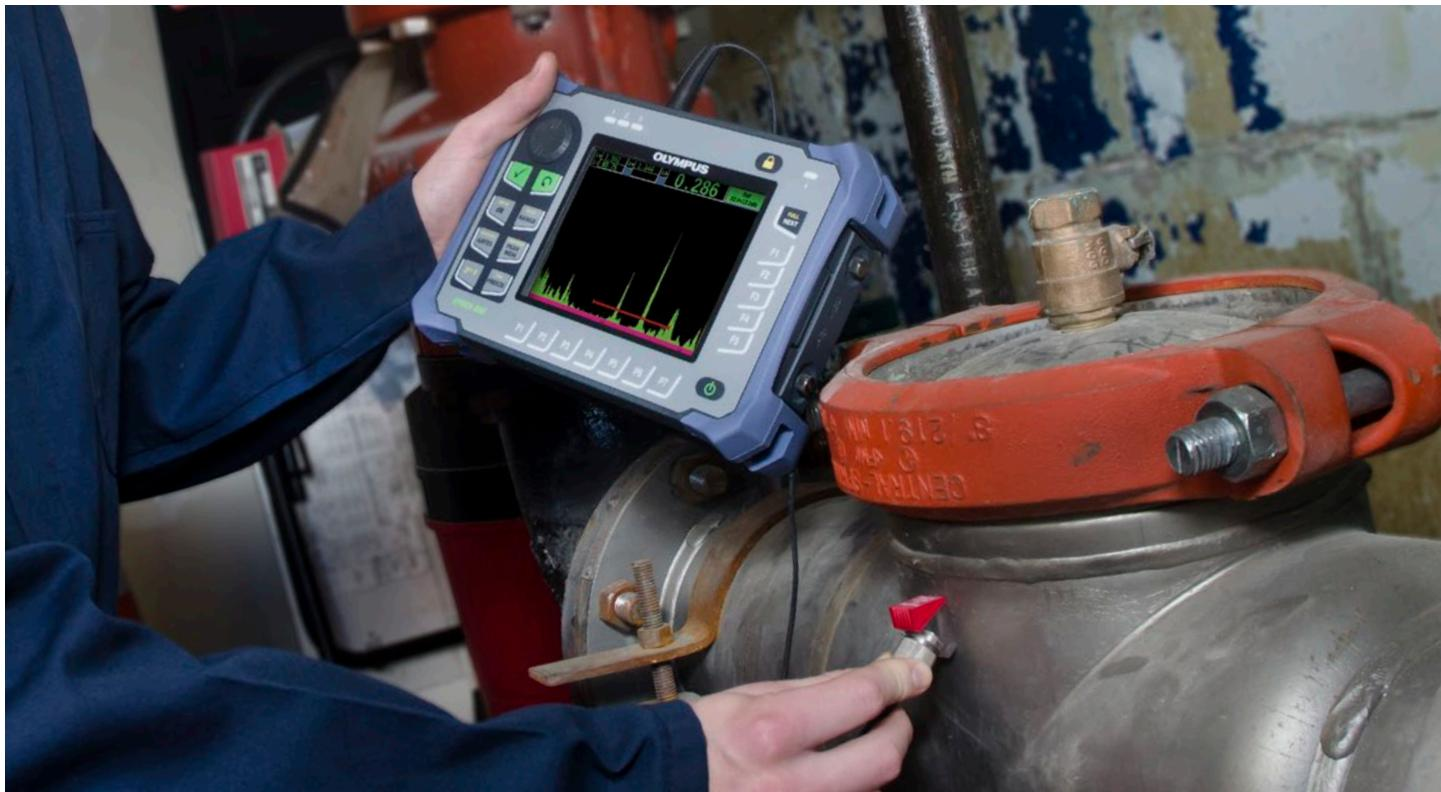
The EPOCH 650 digital ultrasonic flaw detector combines Olympus' industry-leading conventional flaw detection capabilities with the efficiency of a highly portable, intuitive instrument. The EPOCH 650 flaw detector's blend of efficient menus and direct access keys enables you to take advantage of the highest quality flaw detection platform with exceptional ease of use.
